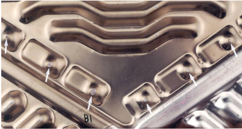
Wear Point Corrosion
